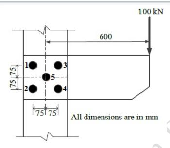
Direct shear on each bolt due to external load,
