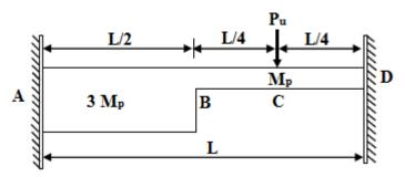
There are two possible collapse mechanisms. In the first mechanism, hinges may form at A, C and D.
