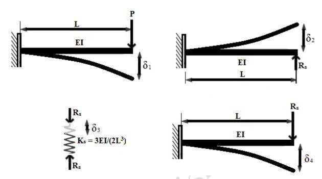
$\delta_1$  = Downward deflection due to load P (causing compression in spring) = PL<sup>3</sup>/3EI
