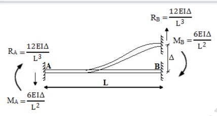
$K_{ij}$  denotes the force in direction i, due to a unit deformation (displacement) in direction j. Thus  $K_{22}$  is the force in direction 2, due to a unit deformation (displacement) in direction 2.
