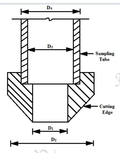
The disturbance of the soil depends on area ratio. The smaller is the area ratio, less is the disturbance.
