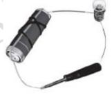
Ans The handle of the screw driver is a bad conductor of electricity and hence does not allow current to pass through it. Thus, the circuit remains open and the bulb does not glow.
